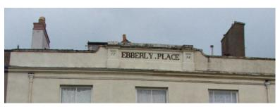
The eastern terrace of Ebberly Lawn features parapet walls that hide the slope of the roof.
